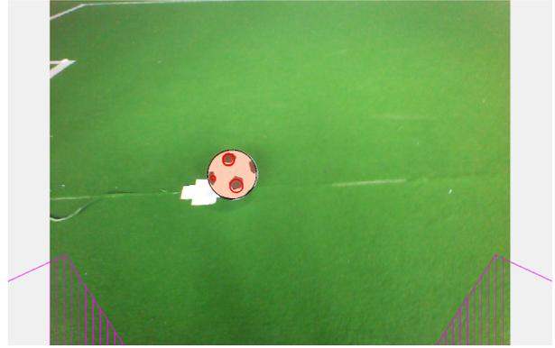
Fig. 2: Detected features on a ball overlapping with the penalty cross.
